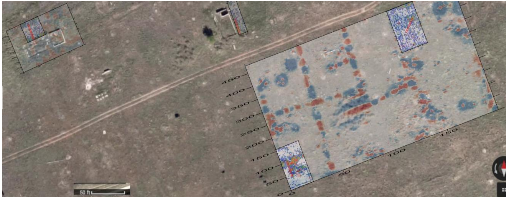
Figure 4-6: Aerial photo of the Industrial Mine Site with magnetometry maps, and ground penetrating radar slice maps. The linear red outlines show the locations of excavation trenches.
