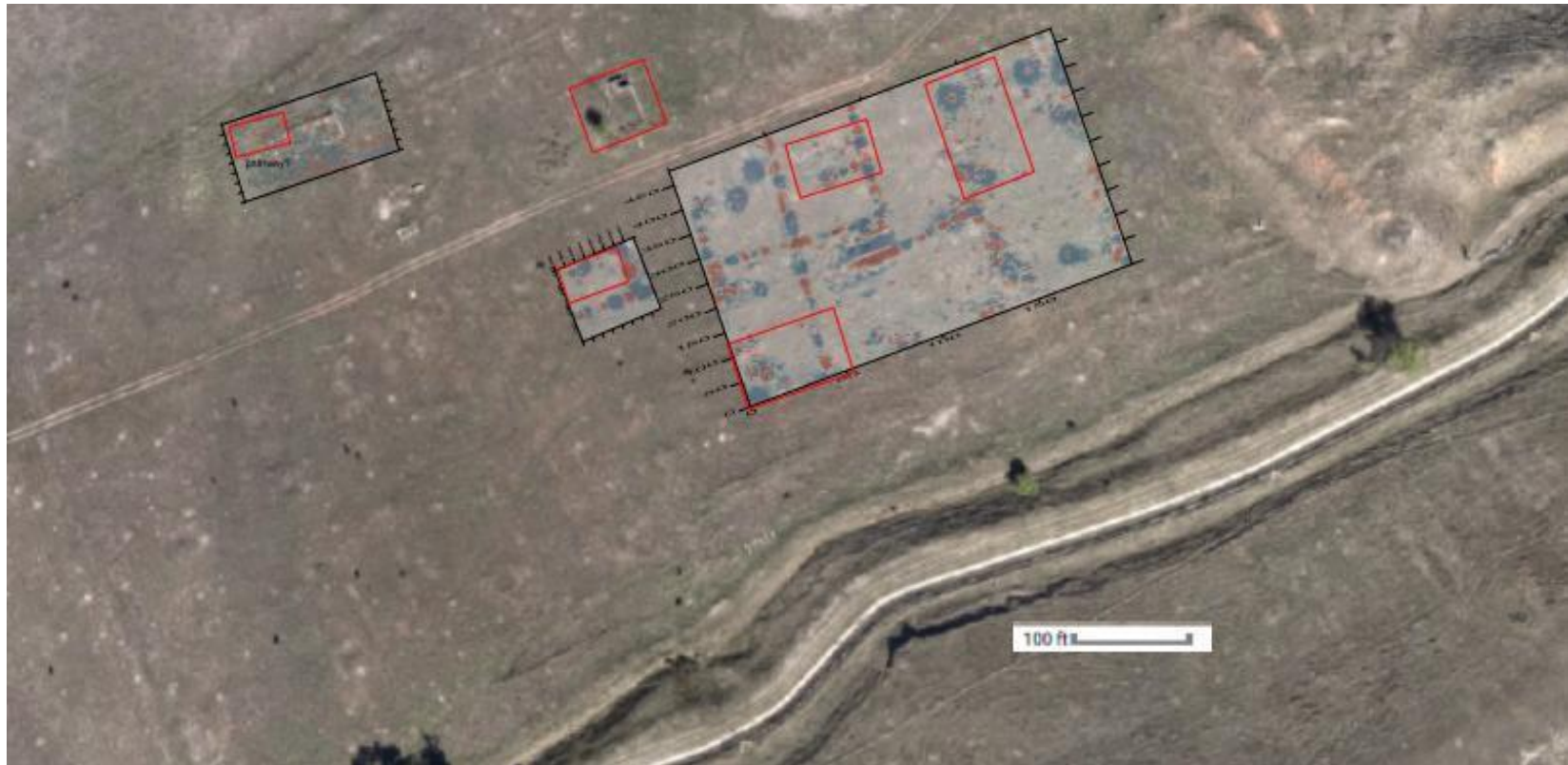
Figure 4-5: Aerial view of the Industrial Mine showing results of a magnetometry survey conducted on the site. The red outlines show the areas chosen for the initial ground penetrating radar surveys.4
